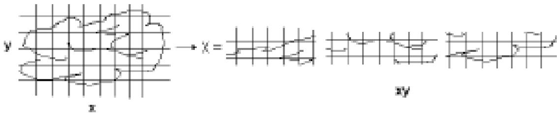
**Fig 2: A row vector representation of a 2-D cloud image**
