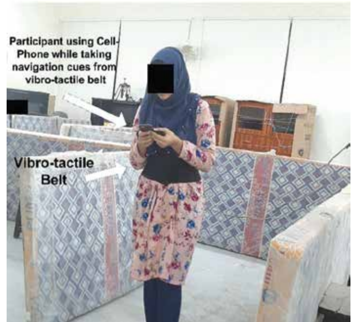
Figure 14: Participant attending to visual display of cell-phone screen, taking the audio commands / white noise from headphones, and taking vibrotactile cues from belt
