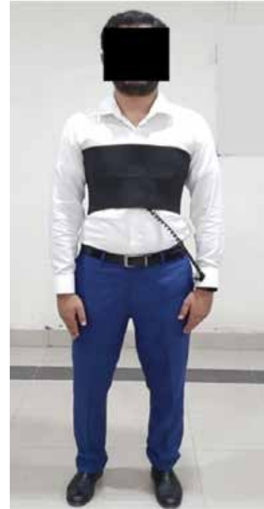
Figure 12: Proposed vibrotactile belt worn by a volunteer
