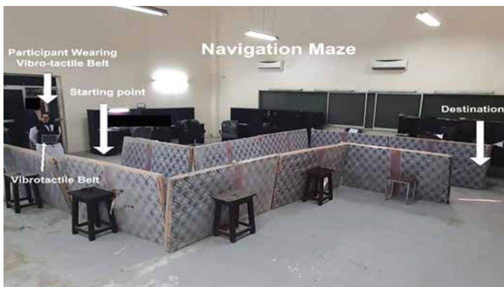
Figure 13: Participant wearing vibrotactile belt in navigation maze scenario while goal of the experiment is to guide the participant to walk through the maze from starting point till end point by taking vibrotactile cues from belt
